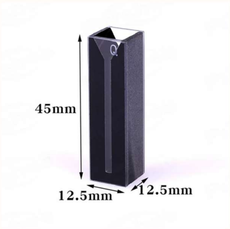
1400µl Slanted Top Quartz Cuvette with Black Walls
