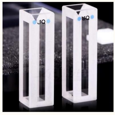
1400µl Quartz Micro Fluorescence Cuvette
