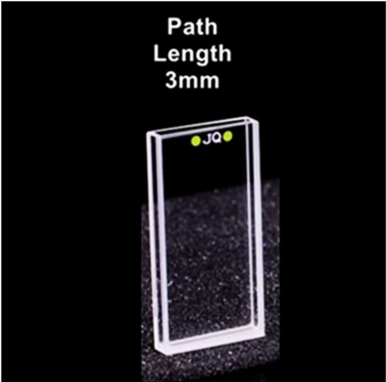
2100µl Quartz Fluorescence Cuvette without Cap
