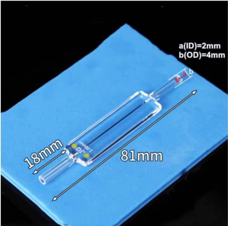
70µl Quartz Flow-Through Cuvette, Path Length 1mm
